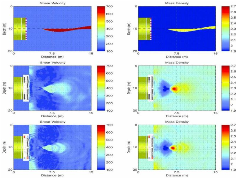
**Figure 1. Numeric scenario with an inclusion to test the full waveform inversion algorithm. Assumed shear-wave velocity and mass-density models and final results are shown. Top row: 2D cross section of the inclusion model. Middle: models after FWI inversion using acquisition Geometry 1. Bottom: inverted models using acquisition Geometry 2.**
