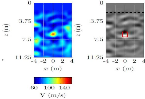
**Figure 3. The pre-processed data and inversion results of the first transect. a) Observed shot gather for a source at  $x = 4$  m. b) Modelled shot gather after inversion. c) Estimated shear-wave velocity model of subsurface. d) Image of subsurface depicting the inclusion. The actual location of the inclusion is marked by the red box.**
