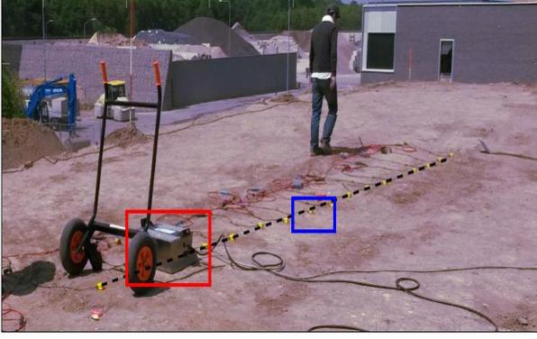
**Figure 5. Field acquisition with the shear-wave vibrator (marked by the red box), especially designed for this application, and the receivers (blue box) along a transect (dashed line) similar to what is typical for a TBM situation.**
